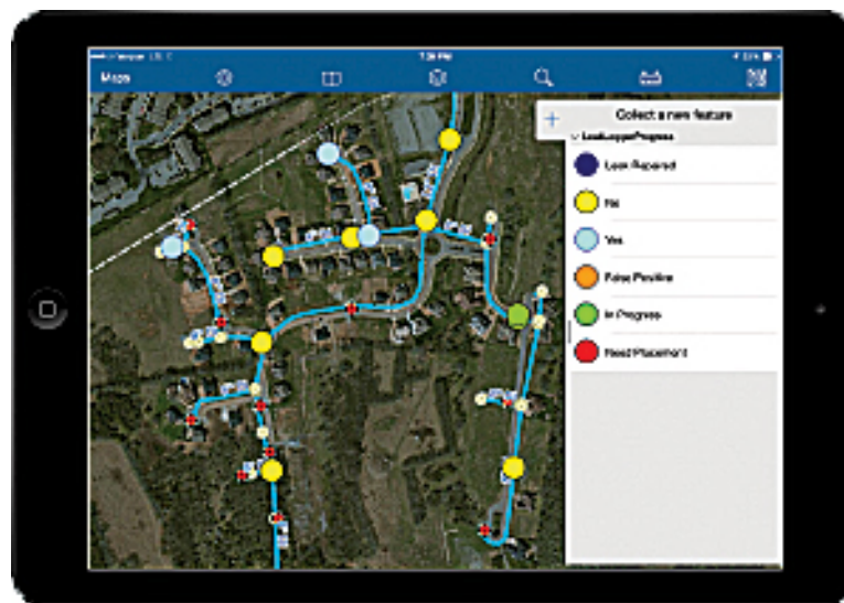
Water Leak Investigator, a solution that is a configuration of the Collector for ArcGIS app, lets field crews pull up detailed information on a specific leak.
